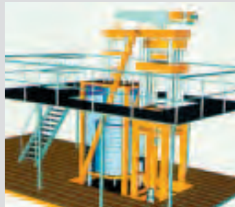
3-D Design of an operating platform
