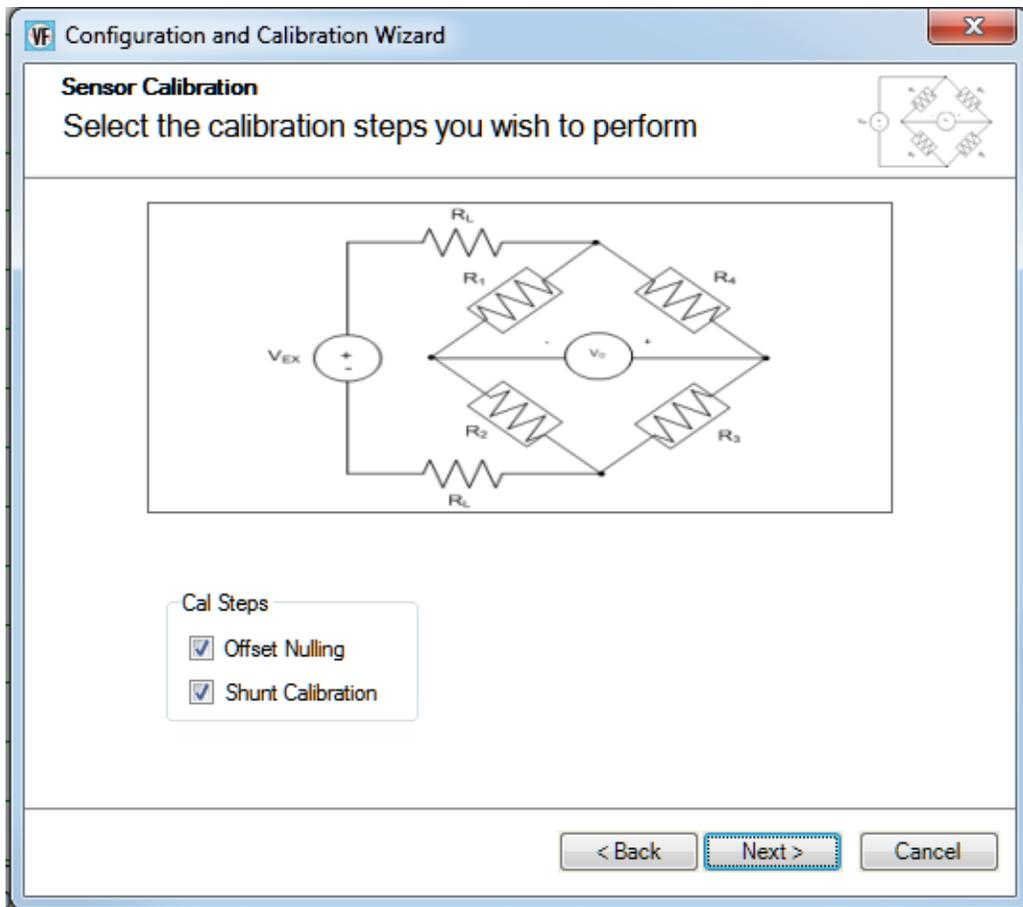
A balanced bridge produces zero volts under ideal conditions with zero strain applied. In practice, however, the output of a bridge in an unstrained condition is offset from zero slightly due to imperfect matching of bridge resistances.
