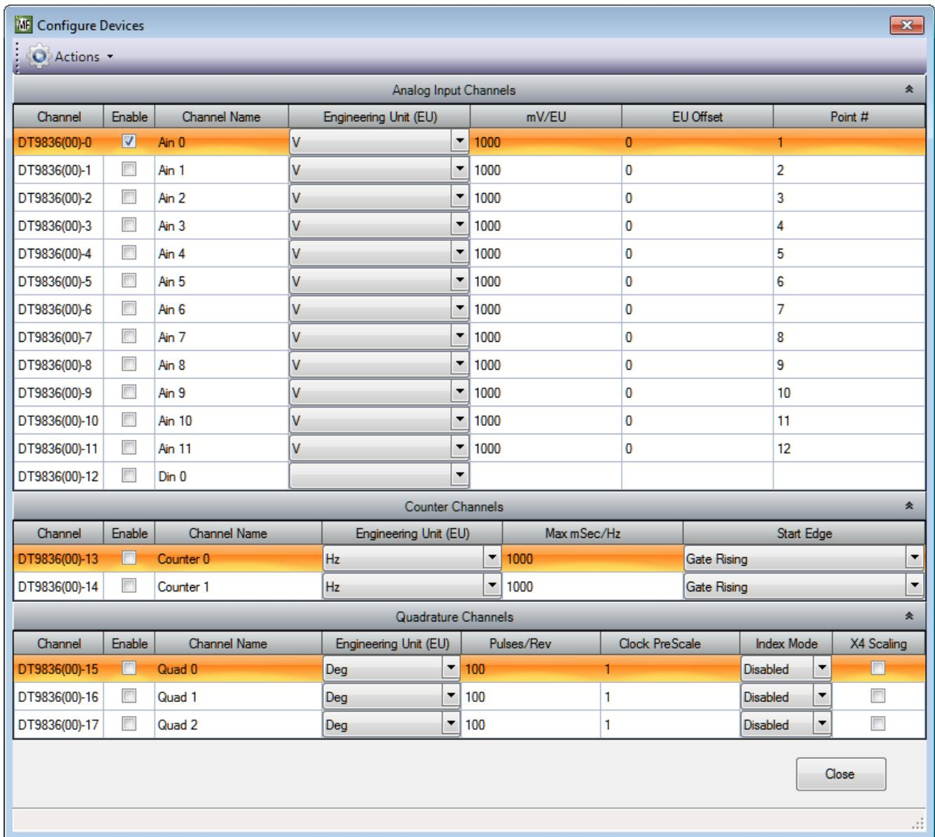
Figure 4: Example Configuration of a DT9836 Module
