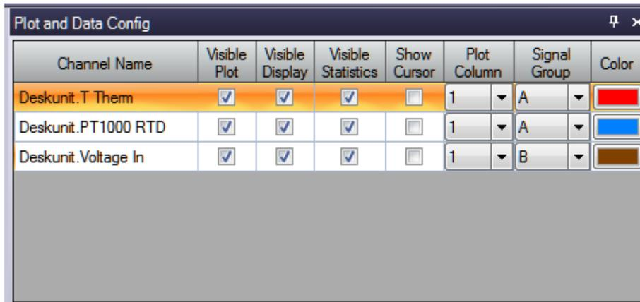
The screenshot shows the 'Plot and Data Config' window with a table of channel settings. The table has columns for Channel Name, Visible Plot, Visible Display, Visible Statistics, Show Cursor, Plot Column, Signal Group, and Color. Three channels are listed: Deskunit.T Therm (red), Deskunit.PT1000 RTD (blue), and Deskunit.Voltage In (brown). All 'Visible Statistics' checkboxes are checked.
