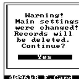
To exit from Programming mode from any Setup page and return to Main Menu, press **MENU** key. A warning message appears, with a confirmation request.
