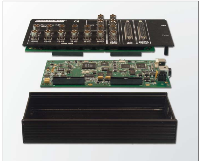
Figure 1. The BNC connection box packages the OEM embedded versions of the hardware in a CE-compliant enclosure.
