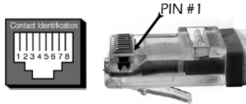
Figure 54: Sync Bus (RJ45) Connector
