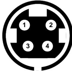
Figure 52: Layout of the DIN Power Connector
