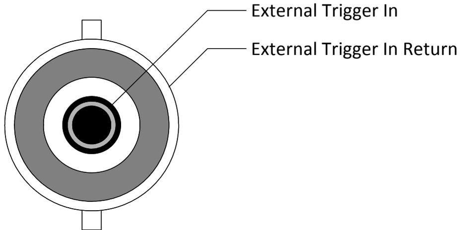
Figure 48: External Trigger Connector (DT9857E Module Only)
