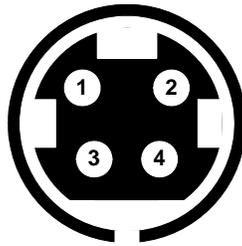
Figure 51: Layout of the DIN Power Connector
