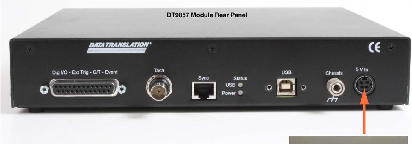
Connect the EP361 Power Supply to the Module and to the Wall Outlet
