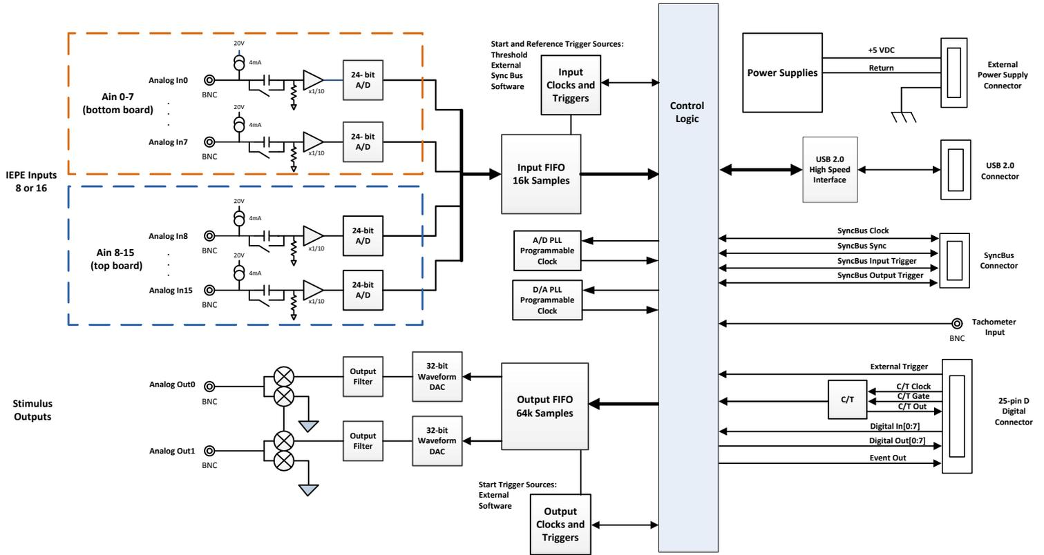
Figure 31: Block Diagram of the DT9857 Module
