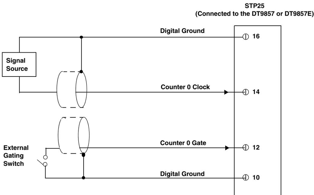
**Figure 23: Connecting Counter/Timer Signals for an Event Counting Operation Using an External Gate**
