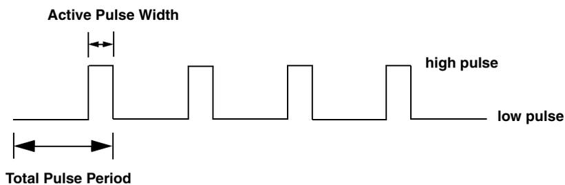
**Figure 35: Example of a Low-to-High Pulse Output Type**
