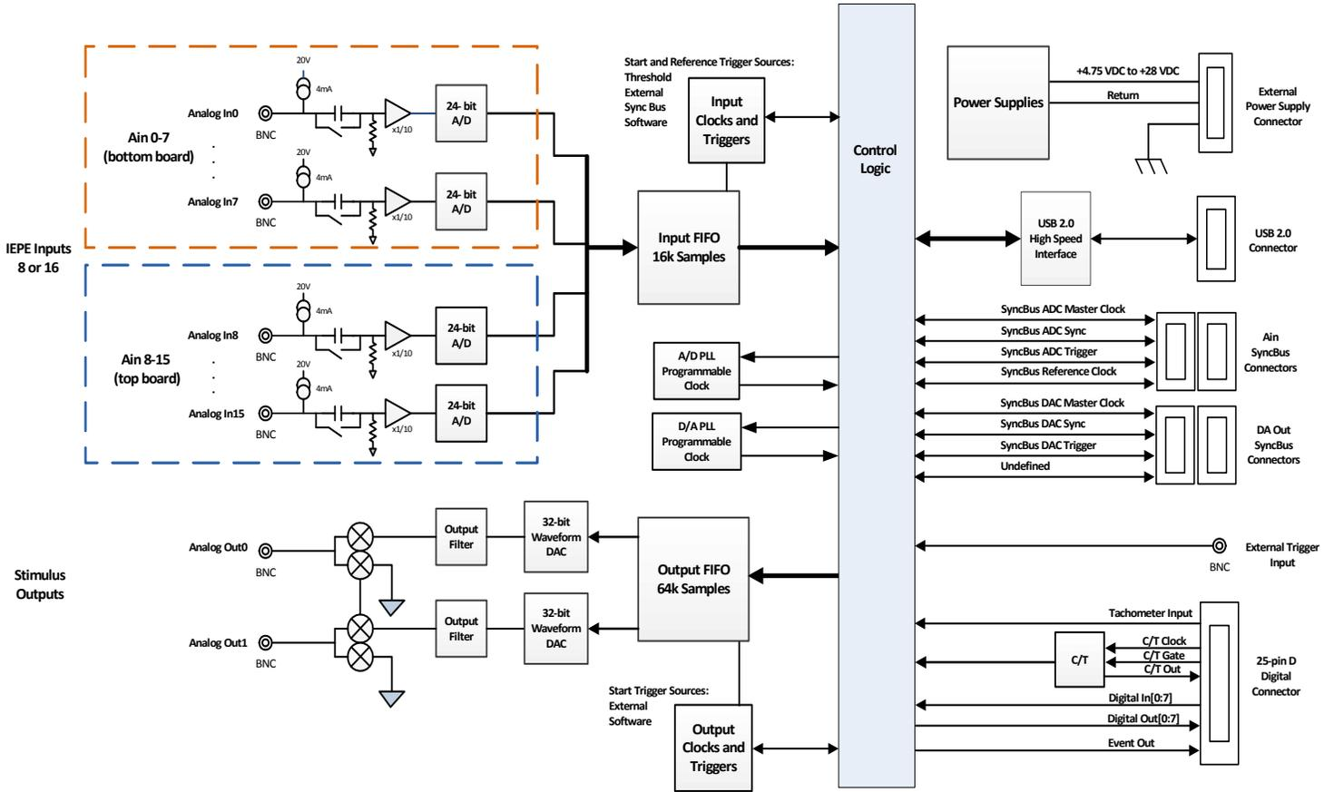
Figure 32: Block Diagram of the DT9857E Module
