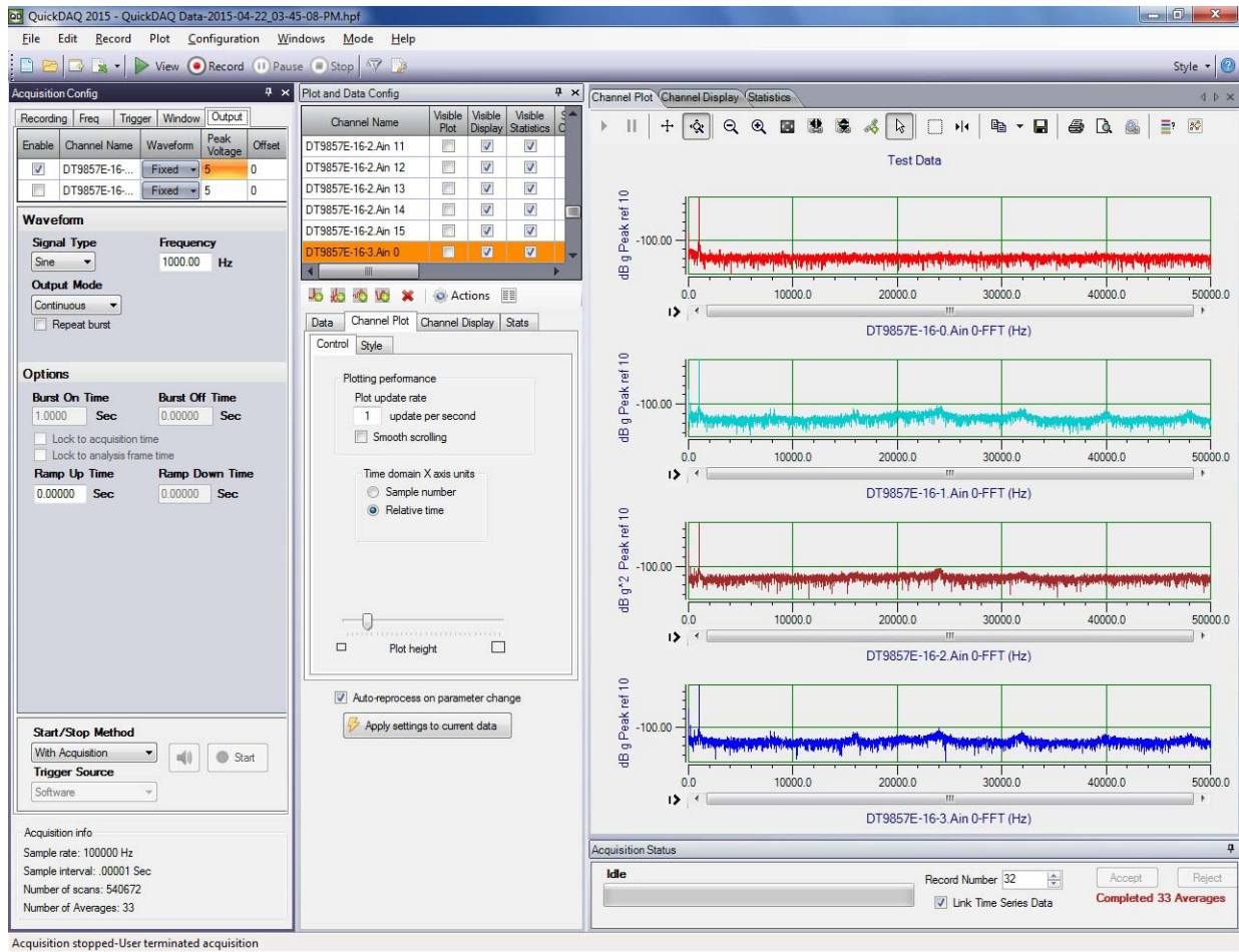
Figure 10: Reduced Performance of 10 dB when the Analog Output is Connected to the Input of a Different Module
