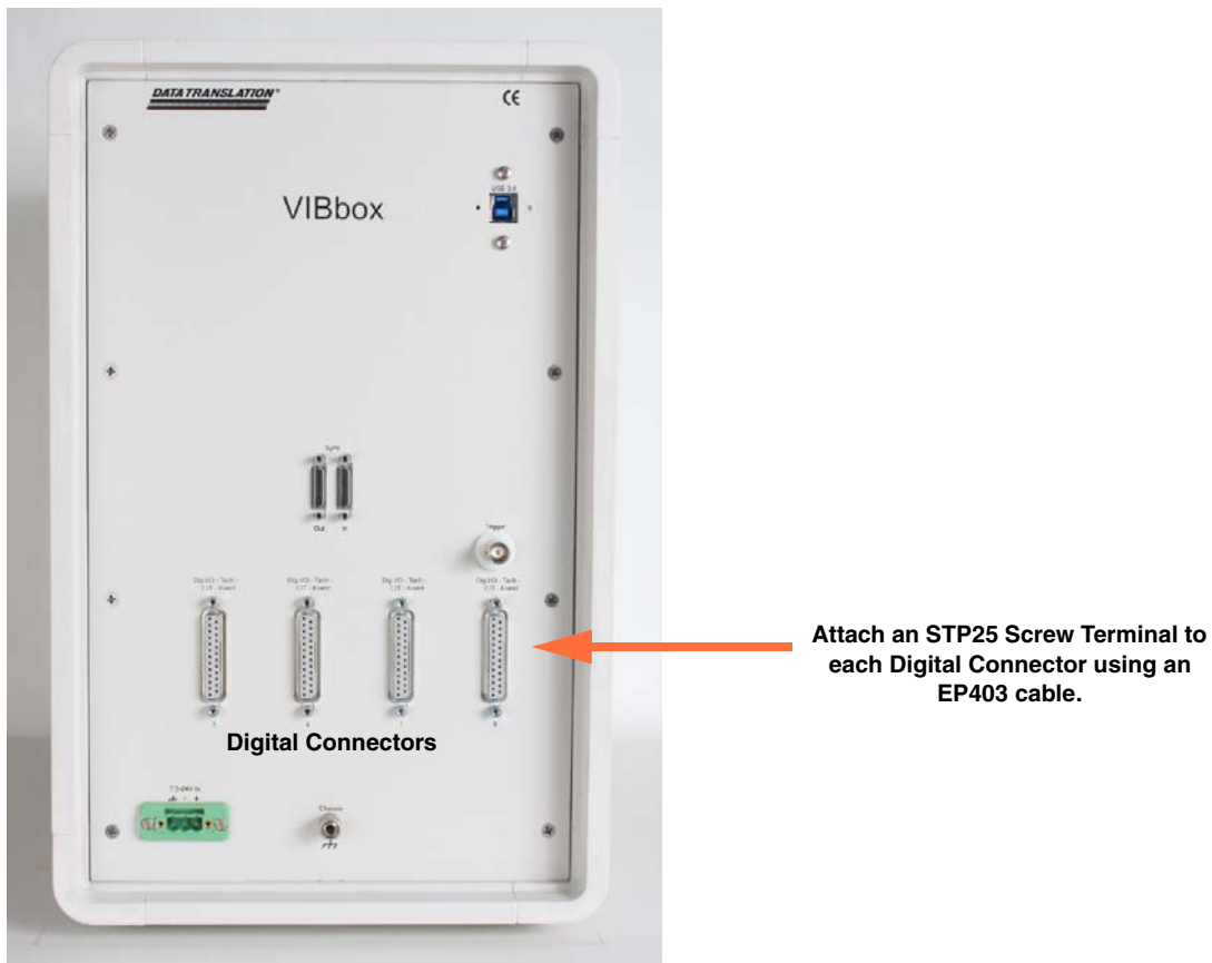
Figure 14: Connecting the STP25 to a Digital Connector on the VIBbox
