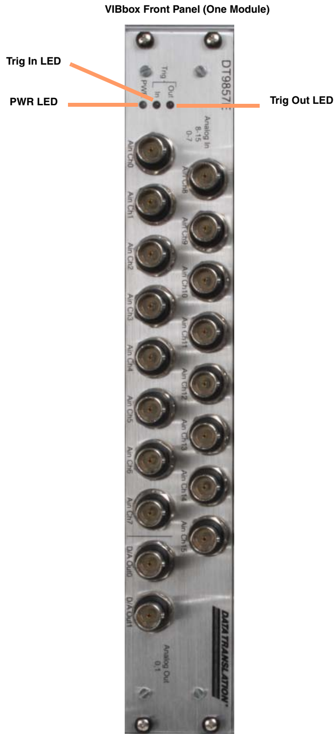
Figure 49: LEDs on the Front Panel of Each Module in the VIBbox System
