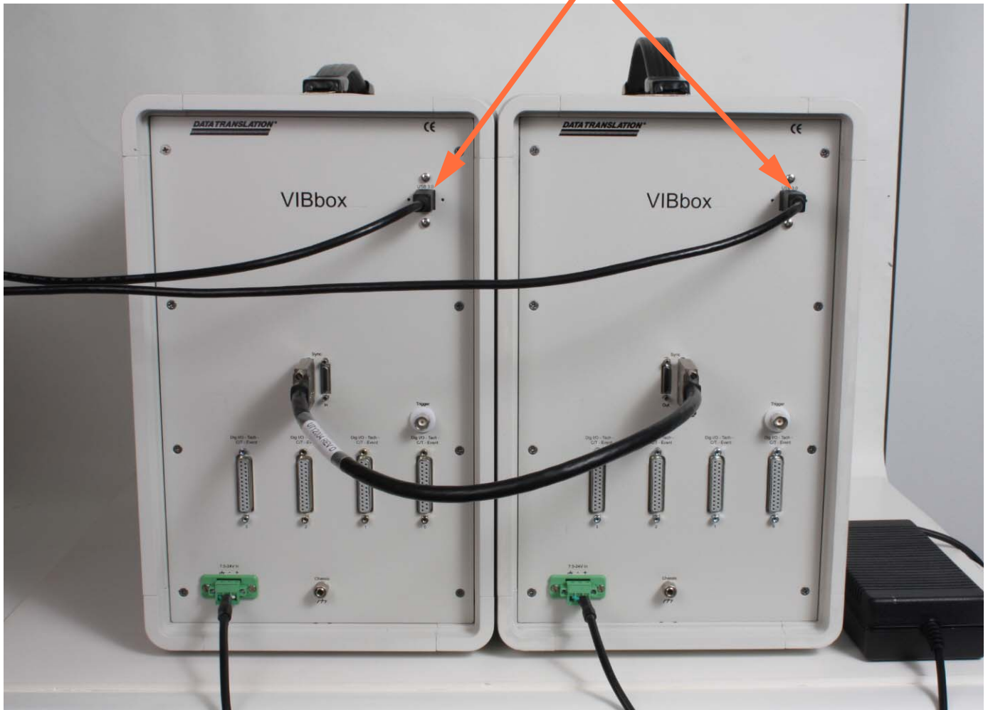
Figure 53: Attaching USB Cables to Each VIBbox
