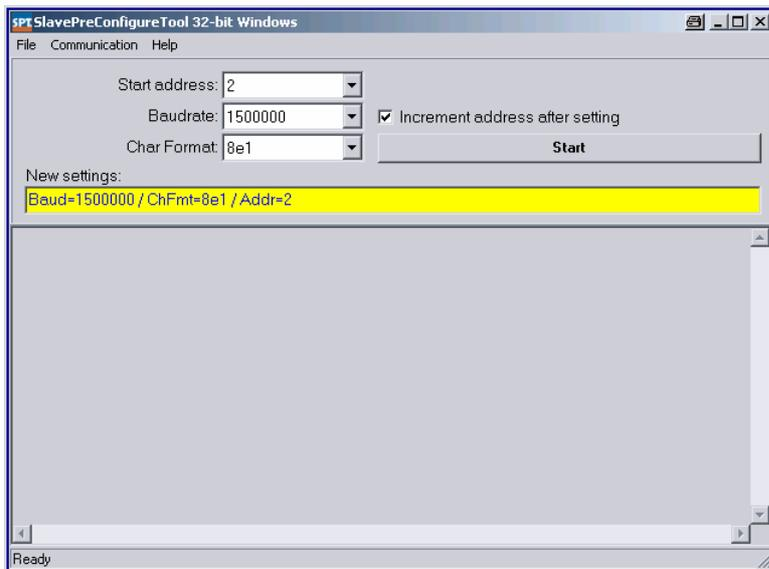
At first the Com Port has to be selected with the function Communication – Parameters .... After that the values for the starting address, the baud rate and the transmission format have to be fixed.
