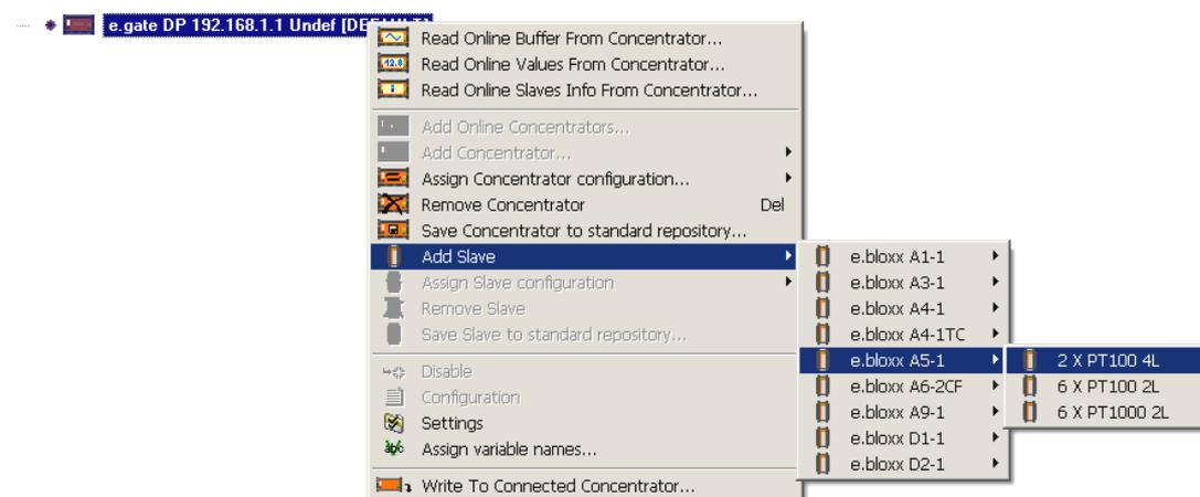
Now the slaves can be added module by module. e.commander is offering a serial line (UART) and an address starting at UART 0, Address 1
