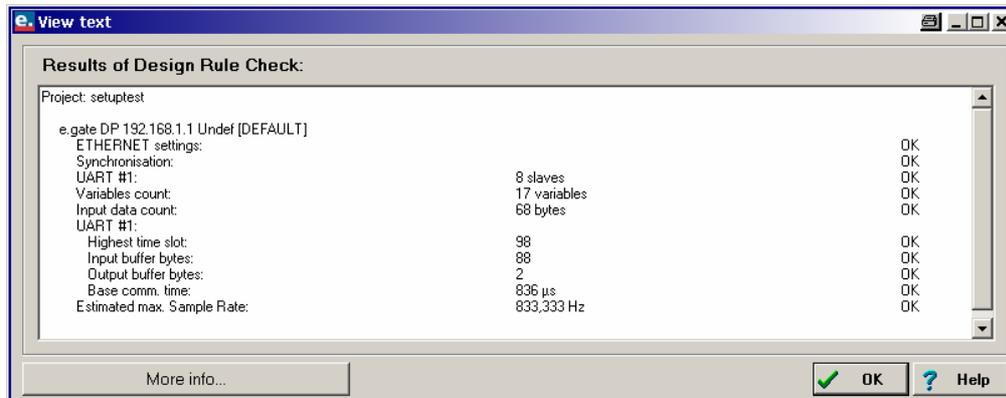
In this case the set-up is OK, there are 8 modules each with 2 channels plus time stamp resulting 17 variables and a sample rate of 833,333 Hz can be reached.
