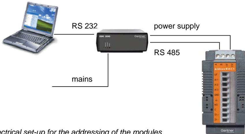
*Electrical set-up for the addressing of the modules*
