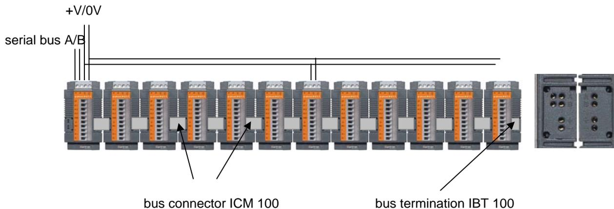
The bus connector ICM 100 connects the serial bus and the power supply between the modules. But due to the power consumption it is not favourable to feed more than 6 modules via the ICM 100. In this case we recommend to connect the power supply direct to the module (see picture above).
