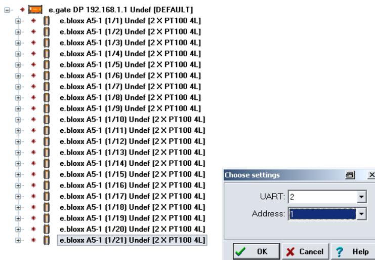
In this way it is possible to set up the whole test stand configuration. In the case that the number of channels increases the maximum numbers of modules in all 4 module lines (UARTS), a further e.gate has to be used. In this case the different e.gate has to be synchronized by connecting I/O 7 and I/O 8 of every e.gate. It is mandatory that the grounds of each e.gate are connected together. For configuration see the e.commander manual.
