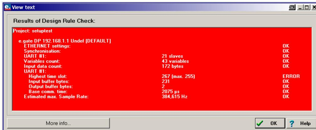
The next required modules can be set to the next line (UART), starting with address 1.
