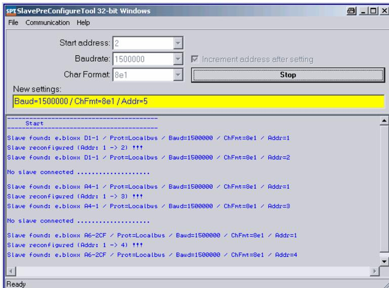
For the second line the procedure is the same. At first select Start address (again 2) and start the process as known. Connect each module of line 2 (example 10 x e.bloxx A4-1) one after the other.
