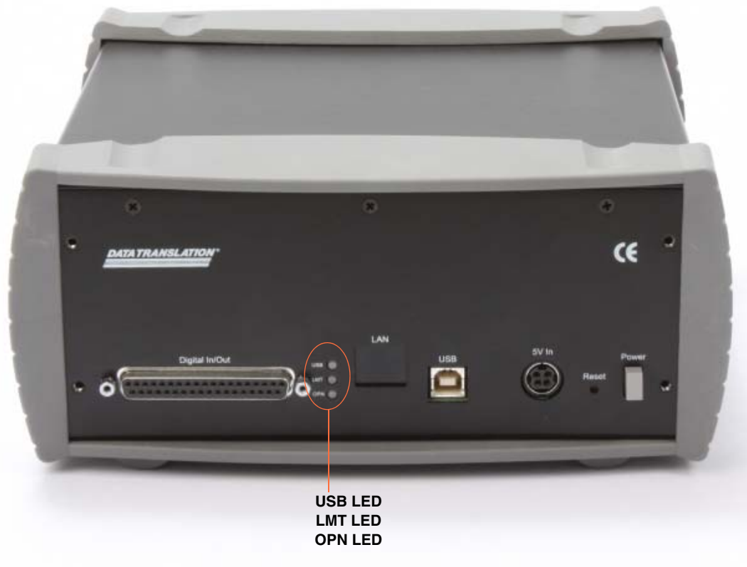
Figure 10: LEDs on the Rear Panel of the Instrument
