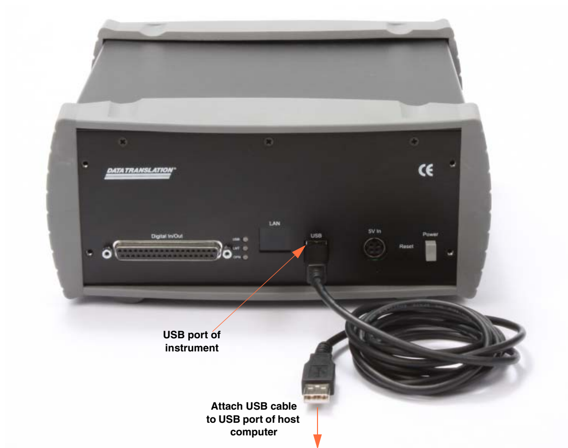
Figure 9: Attaching the Instrument to the Host Computer
