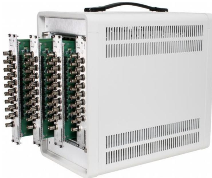
**Figure 2.** VIBbox-64 packages four DT9857E modules in a rugged enclosure for field use. The user can take advantage of the full expandability of this module series in a self-contained enclosure. The use of a USB hub internal to the system allows easy connection to the host computer through one simple USB cable. An external power supply is included.
