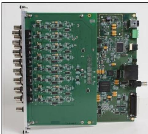
**Figure 3.** The DT9857E provides sixteen IEPE analog inputs, 2 analog outputs, 16 DIO, 1 C/T, 1 Tachometer, and 2 Measure Counters on each board set. VIBbox-64 packages four of these to bring the channel count to: 64 IEPE analog inputs, 8 analog outputs, 64 DIO, 4 C/T, 4 Tachometers, and 8 Measure Counters. For more information on the DT9857E module, visit our web site: <http://www.datatranslation.com/products/dataacquisition/usb/DT9857E/>
