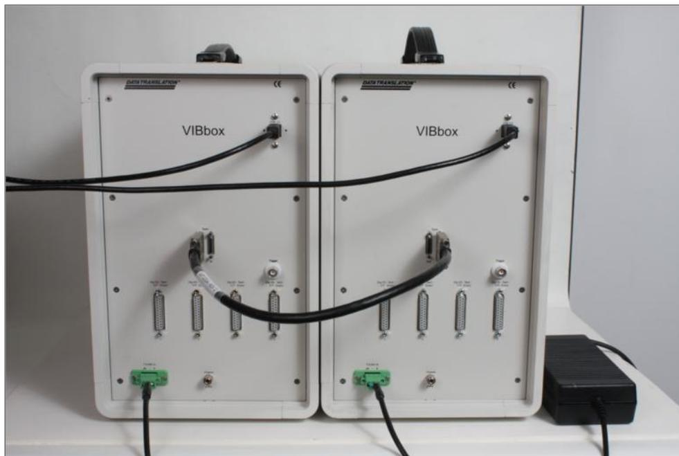
**Figure 4. Multiple VIBboxes can be connected together (two VIBboxes shown here) using one or more EP377 Trigger Bus cables. Each VIBbox must be powered using an external power supply and connected to the USB 3.0 port of the host computer.**
