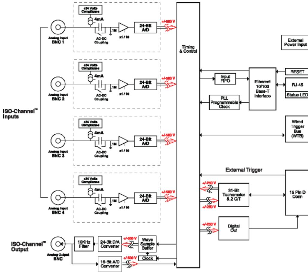
Figure 18: Block Diagram of the DT8837 Instrument Module
