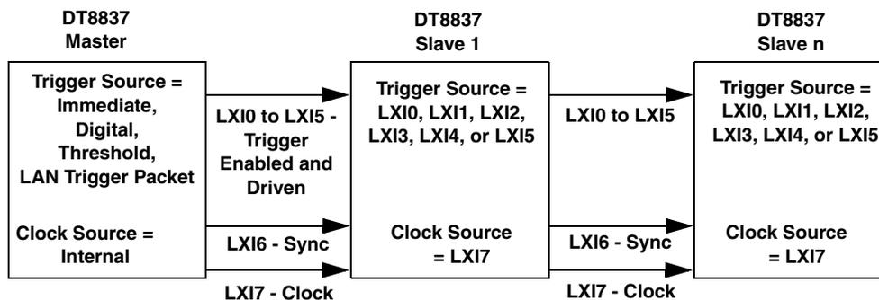
**Figure 21: Synchronizing the Start of Acquisition When Connecting Multiple Instrument Modules to the Trigger Bus**
