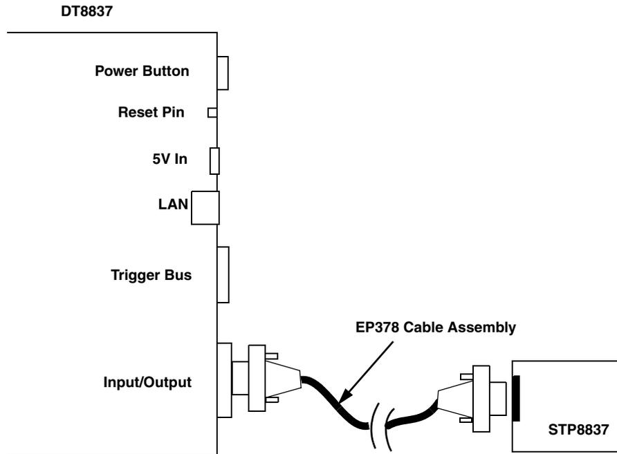
**Figure 12: Connecting the Instrument Module to the STP8837**
