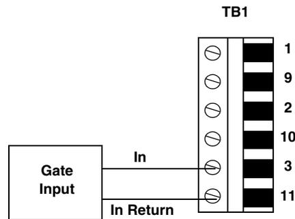
**Figure 15: Connecting a Gate Input Signal to the STP8837**
