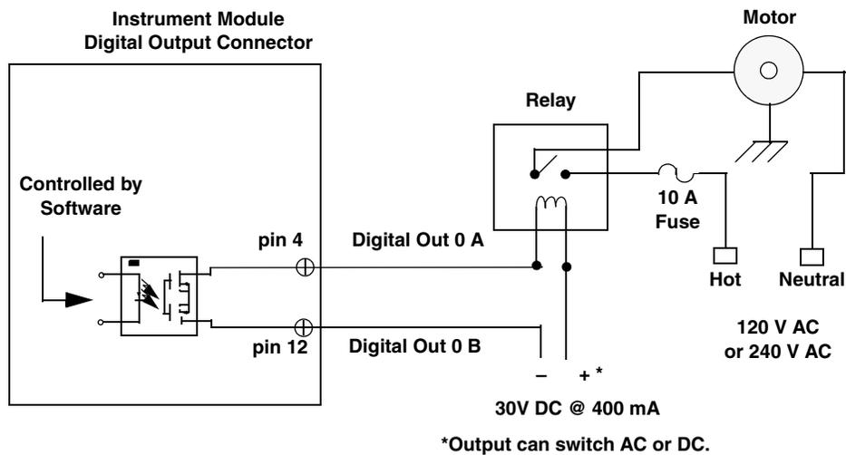
Figure 16: Switching up to 30V at 400 mA
