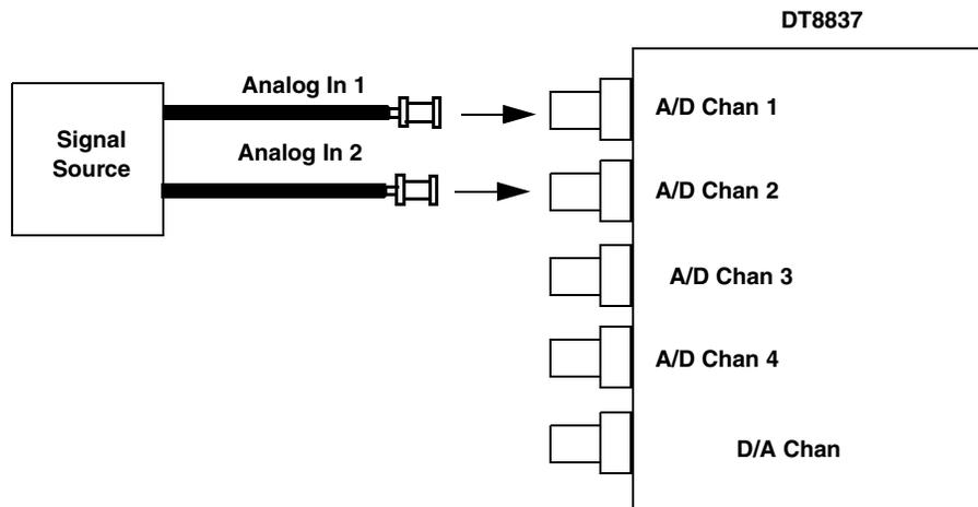
**Figure 10: Connecting Analog Inputs to the DT8837**
