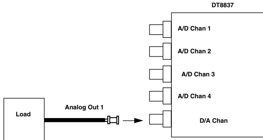
Note that the BNC automatically connects the Analog Ground signal appropriately.
