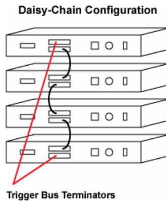
**Figure 20: DT8837 Instrument Modules in Daisy-Chain Configuration**
