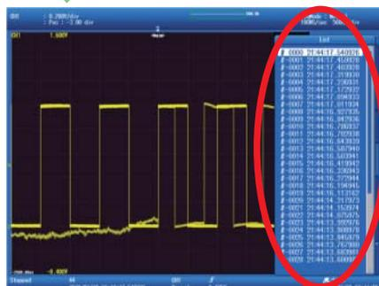
You can display all past waveforms, and view a list of acquisition times at min 1  $\mu$ s resolution
