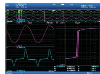
Magnetic flux density:  $B = \text{Integ}(C1) / (K1 \cdot K2)$
