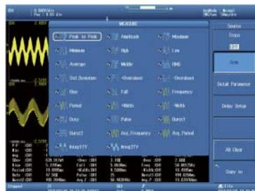
Detect abnormal waveforms, notify users, and determine pass/fail — GO/NO-GO determination —
