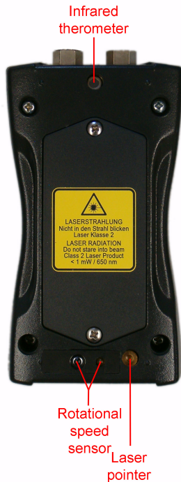
Figure 34: Rotation speed and temperature sensor, laser pointer
