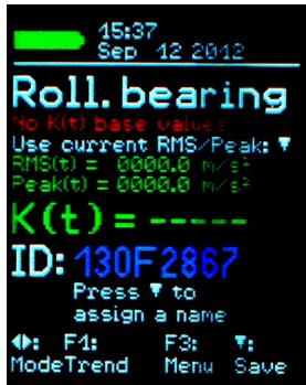
Figure 27: K(t) mode with newly detected VMID
