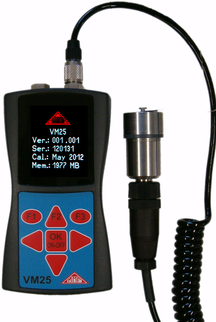
Figure 1: VM25 with vibration sensor
