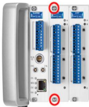
Fig. 4-74 To remove a module release the screws in the blue circles on the rear panel.
