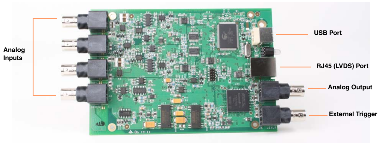
Figure 12: Connectors on the DT9837C-BNC Module
