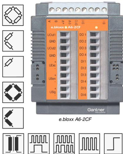
The e.bloxx series is designed for industrial and experimental test systems requiring precise high speed measurement of electrical, thermal, and mechanical quantities in engine and component test beds.
