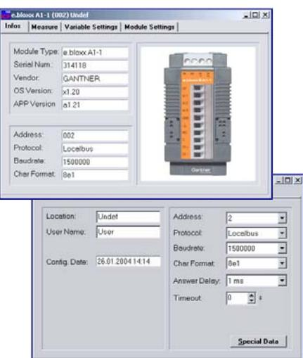
ICP 100 is a 32-bit application for Windows® 95, 98, 2000, NT and XP to configure the e.bloxx series and the ISM series modules
