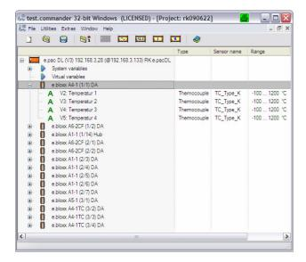
test.commander is a program for Windows<sup>®</sup> 2000, NT, XP, and Vista, which allows complex systems, consisting of one or more Test Controllers and multiple Q.bloxx or e.bloxx modules, to be configured and adapted to the specific requirements.
