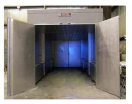
low for batch processing, where materials are loaded onto rolling carts, positioned in the oven, cured, and then rolled out. Characterizing and optimizing the curing cycle is critical in controlling the final properties of the composite material.
