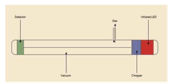
Infrared light is sent through the two chambers, one with the gas and one without (a vacuum). The detector compares the two to determine how much gas is present.
