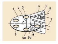
The light gets interrupted by the chopper wheel and the detector induces a voltage that looks like the graph.
